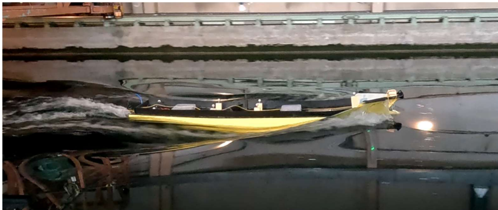
Figure 2.12 Frame of the recording of the calm water speed calibration in the CTO towing tank
