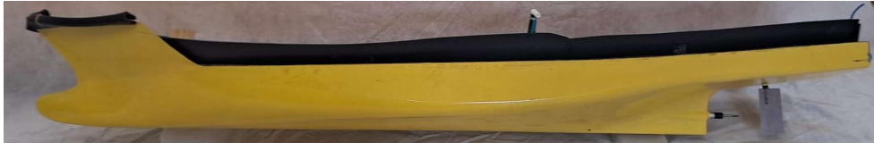
Figure 2.3 Radio-controlled self-propelled model of the ITTC A2 purse-seiner manufactured in 1/14 scale
